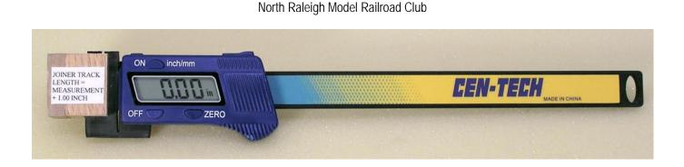
Above is a picture of an easy-to-make gauge that greatly reduces the amount of time it takes us to install joiner tracks at NTRAK meets. This has been used for over 4 years, and it has proven to be very reliable and easy to use.
