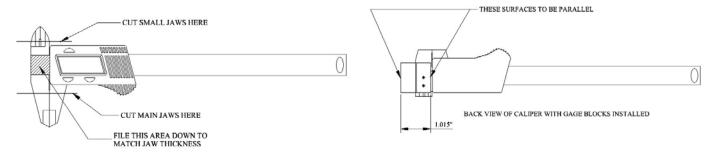
The width of the wooden gauge blocks should be around 1". The following pictures show the geometry and location of the gauge blocks.
